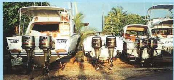
High horsepower outboards used in tandem are popular now with private pleasure boat owners.
