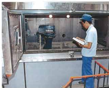
Endurance-testing an outboard with the company's original complex-corrosion test machine
