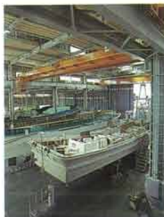
Large-size fishing boats along with pleasure boats are built in the 4th plant.
