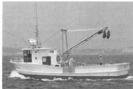
Through a 1988 JICA project to the Republic of Cape Verde, this dual-purpose boat was sent for use in both purse seining and pole and line fishing.
