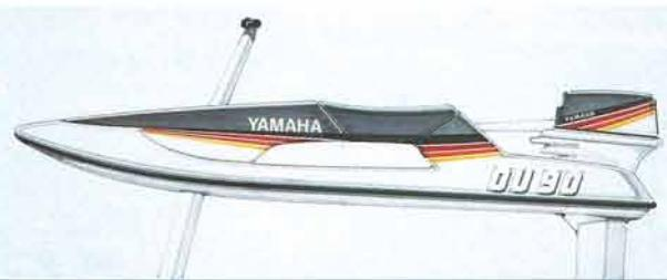
An open hydrofoil boat 'OU-90' which was exhibited together with the OU-32 at the Expo 88 Brisbane, was a single-seater model powered by a 15hp outboard motor.
