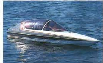
*A dream sports boat 'OU-32' rises and cruises above the water by means of lift force working on its underwater foils.*
