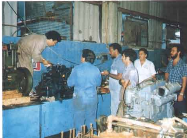
An engine is being disassembled for technical inspection (Cuba)
