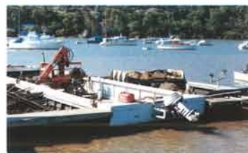
Oyster punt with crane for lifting racks
