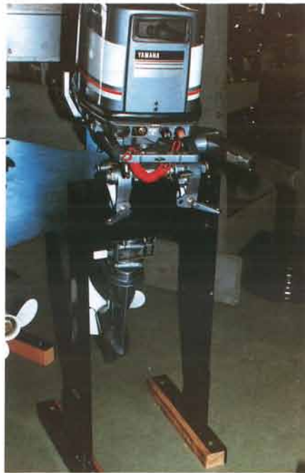
This is a stand for a small-horsepower outboard which was made from the packing materials for a large-horsepower engine.
