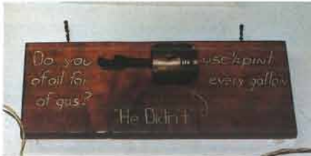
An example of a seized piston hanging on the wall of Buck's workshop. Beside it is written; "Do you use 1/2 pint of oil for every gallon of gas" (16:1 mixture ratio)
