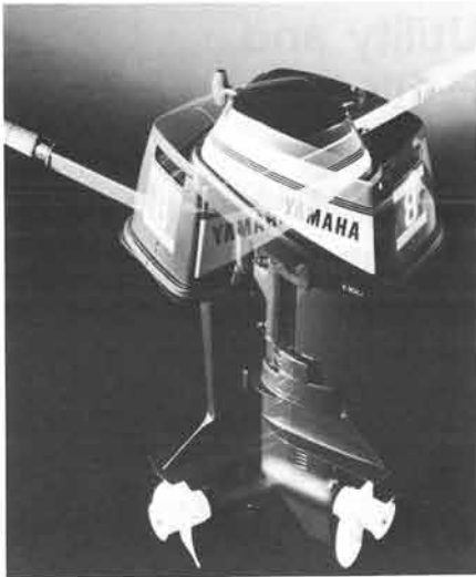
Fig. 4. Steering handle has a steering angle of up to 120°
