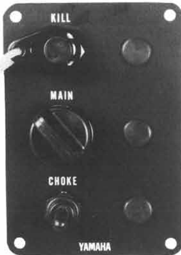
Switch panel. Seen on the left end is a kill switch.
