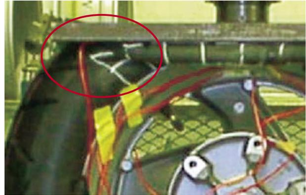
Fig. 11 Shape of compressed tire in static test
