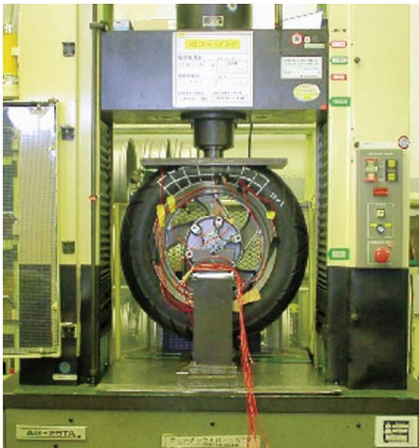
Fig. 8 Tire compression test overview
