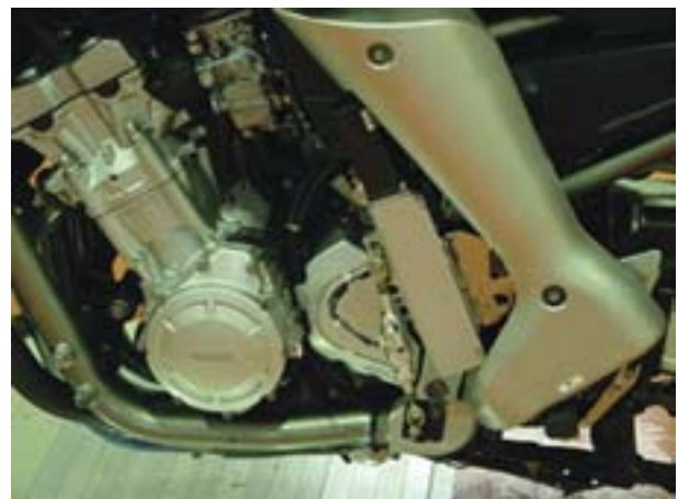
Figure 11 New-type shift load sensor mounting status
