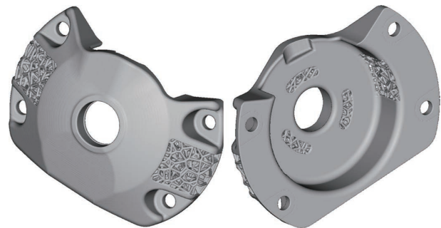
Fig. 14 Final shape including lattice structure
