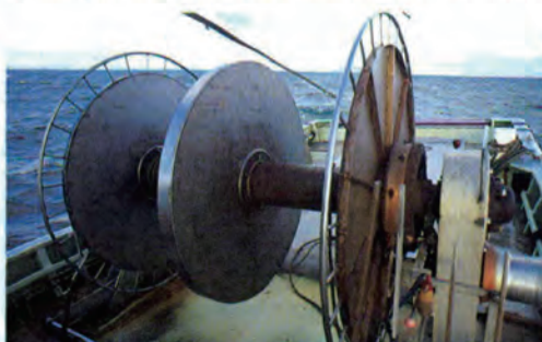
(Above) A net hauler. The drum is divided into two sections, one for winding in the lead rope (left) and the other for the net. (Right) When hauling, the net is wound in as far as the wing net.
