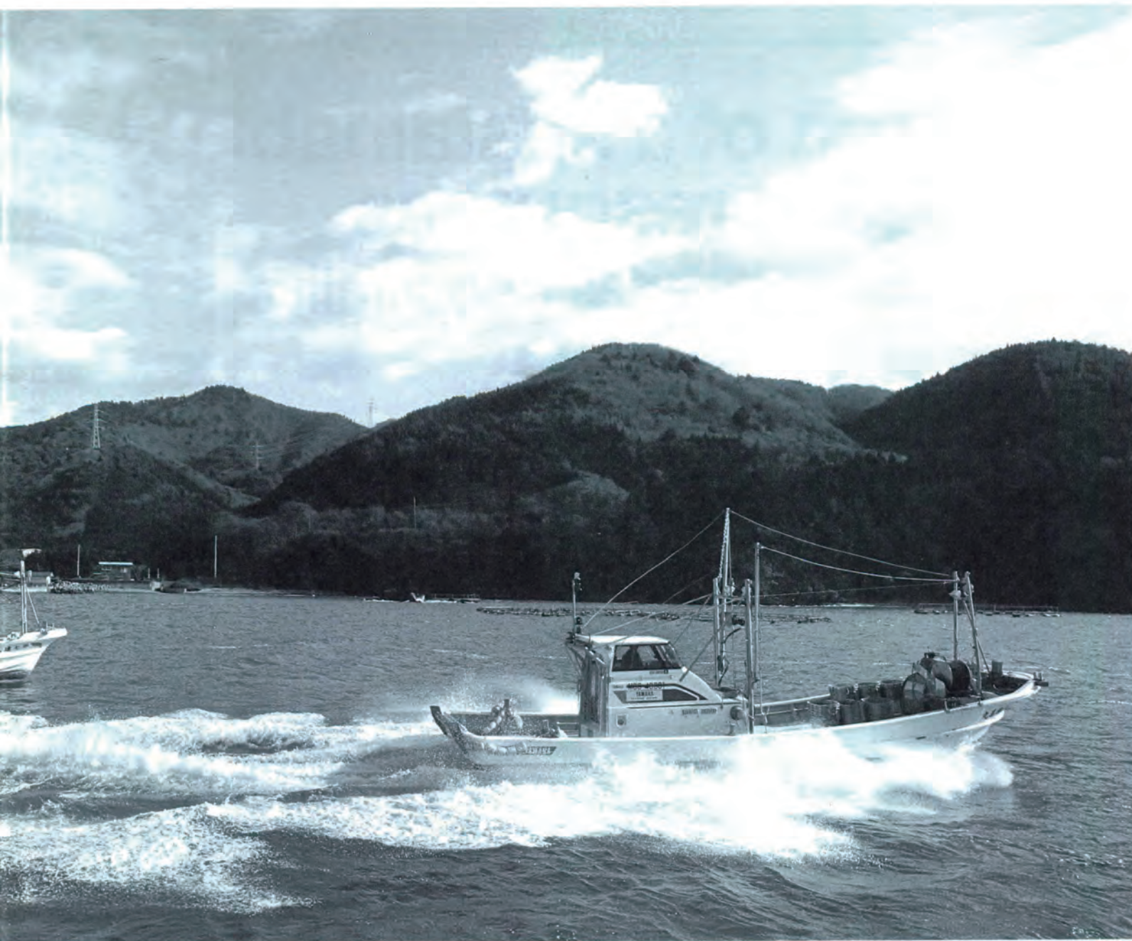
Roughly 300,000 small-class fishing boats are at work today in Japanese coastal fishery. Most common among these are diesel-powered 1-3 ton and 3-5 ton boats, making up some 40% of the total. Fishermen choose the most suitable type of boat based on the fishery they engage in and the size of their operation. At the same time, there has been a growth in 1-ton class utility boats motorized by means of outboard motors. These boats are employed largely in shellfish and seaweed gathering operations and aquaculture in shallow water areas.
