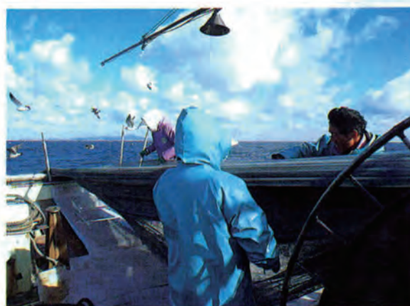
(Above) A net hauler. The drum is divided into two sections, one for winding in the lead rope (left) and the other for the net. (Right) When hauling, the net is wound in as far as the wing net.
