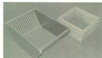
Selection (sorting) sieves. The fish are sorted out according to the gauge of the wire mesh or the spacing of the rods. Six or seven such sieves with different mesh dimensions are prepared.
