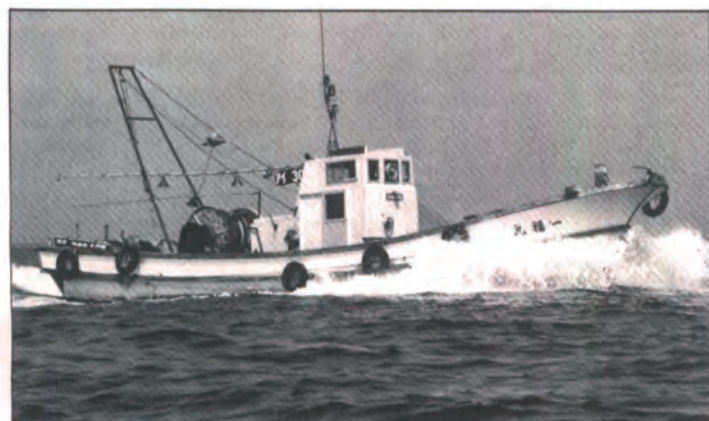
Yamaha DT-46-0A. The same type as an octopus fishing boat for Australia
