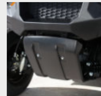
Skidplate for non-extreme off-road protection.
