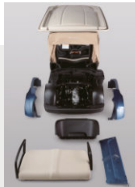
Removable modular body panels to lower costs for maintenance and damage repairs.
