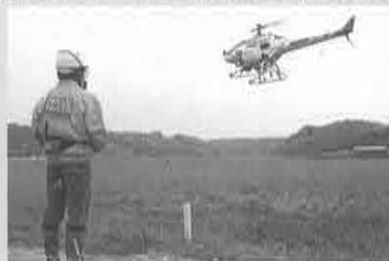
The Yamaha Aero Robot "RMAX" made its debut in October 1987, mounting a specially developed horizontally opposed liquid-cooled 2-stroke 241cc engine rated at 21 hp. This made possible an effective
