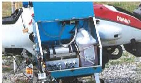
The navigational GPS system is housed in the box on the right side of the helicopter. Next to it is an auxiliary fuel tank
