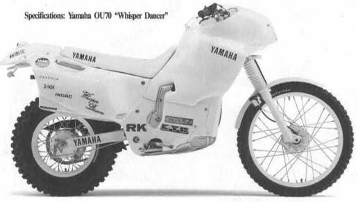
●Engine: Liquid-cooled 2-stroke 200cc ●Wheelbase: 1,367mm ●Seat height: 830mm ●Minimum ground clearance: 268mm
