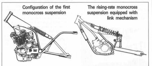
sion system; one that functions with a rising-rate effect that changes with the strength of the shock encountered.
