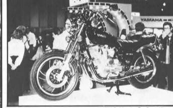
The entirely-new DOHC 4-cylinder XJ650G Maxim I. Specific attention is called to the shaft-drive system and aluminum cast wheels.
