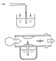
Air pressure within the cylinder (crankcase in case of a 2-stroke engine) becomes lower than normal atmospheric pressure during the intake stroke.
