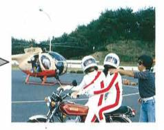
A new '80 racer! No, don't jump to any hasty conclusions. This is a pocket bike designed and marketed by Sunward International Inc. in Japan. As you see, the bike is an imitation of the GP-winning YZR500. The overall length is 925mm and the total weight is 16Kg! Powered by a 1.6PS 2-stroke 30.5 cc engine and fitted with both 3.00-4 in. tires, the bike can carry even an adult rider. The bikes of
