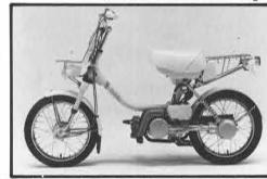
The nicely styled Yamaha MA50 50cc looks like a nimble sportcycle. An automatic transmission gives a quick, positive response. A newly designed muffler lowers noise level. Seat height is 695mm allowing easy footing.
