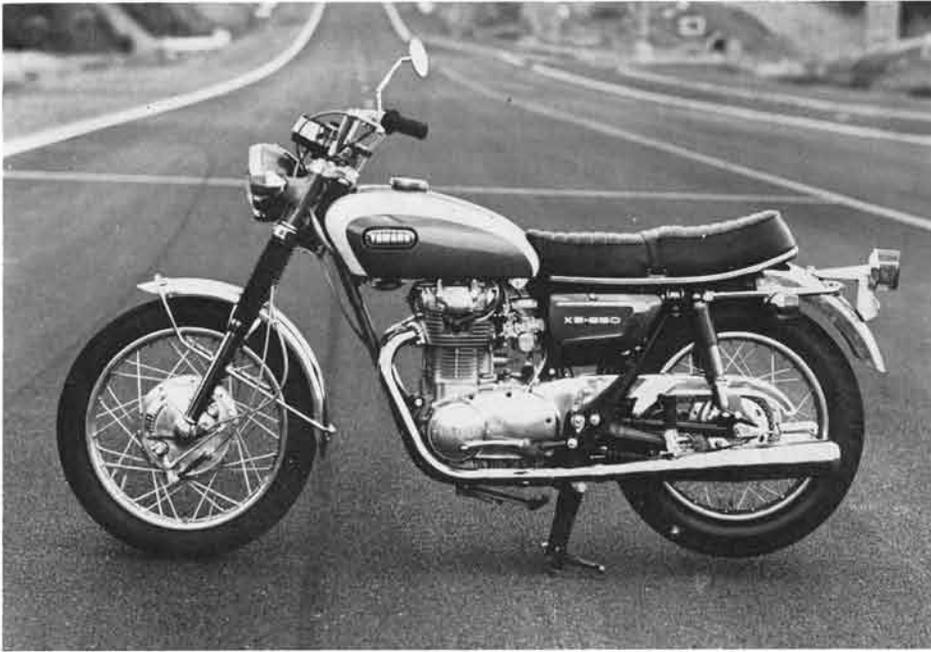
A maximum output of 53 h.p., acceleration of 55 1/3 sec. for 1/4 mile, top speed of over 185 km/h, these are figures specified in its technical data for the domestic market. They are far above the standard levels.
