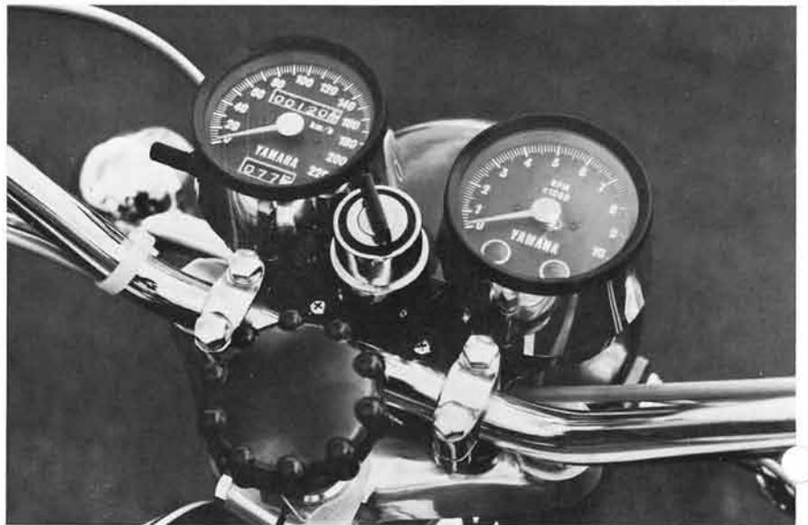
Newly designed speedometer (left), tachometer (right) and ignition key (center).
