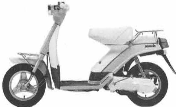
The newly designed stepthrough chassis allows even a novice rider to place either foot on the ground freely whenever necessary. Getting on or off the bike is quite easy. Both carriers are standard equipment.
