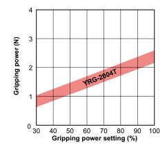
Graph shows a general guide to gripping power versus gripping power setting (%). Variations will appear in the actual gripping power
