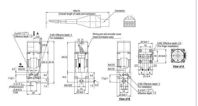
Note. Avoid extreme winding of the cable and fix the cable securely so that it does not move.
