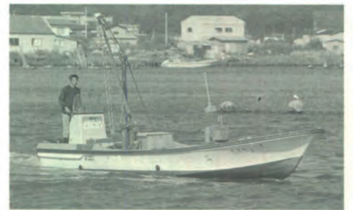
Under 3-ton class workboats are used for smallscale culturing operations. Pictured here is a Yamaha drive boat, YDW-27 (1.3 tons) designed specifically for small-scale culturing. Seen on deck are a simple manual winch and a shell grinder.
