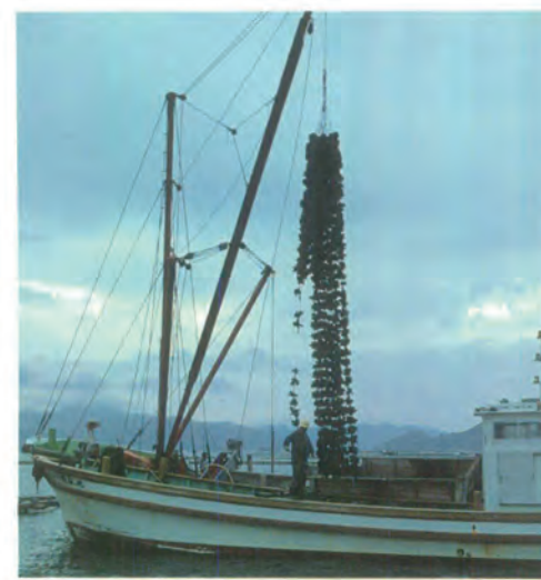
The size of an oyster culture workboat is limited to under 20 tons. The transport boat is equipped with a crane. The foredeck is a full open hold type.
