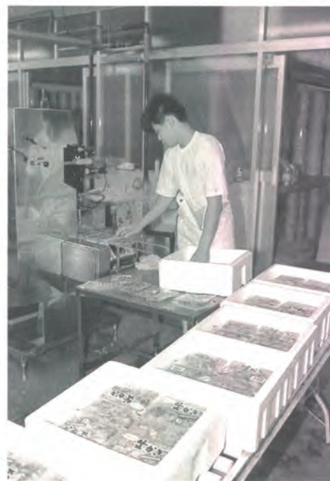
A fresh oyster packaging factory which is run by local middlemen in the producing area. Oysters which are supplied by producers are washed and grouped into three size classes, small, medium and large, with the exception of 'Mizugaki' and egg-bearing oysters before they are automatically sealed into small transparent plastic packs. These packs are ice-packed in styrofoam boxes for shipment.
