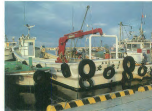
A Yamaha fishing boat used for shrimp pot fishing and scallop culture fishery. On the rear deck is a derrick used in scallop culture operation.
