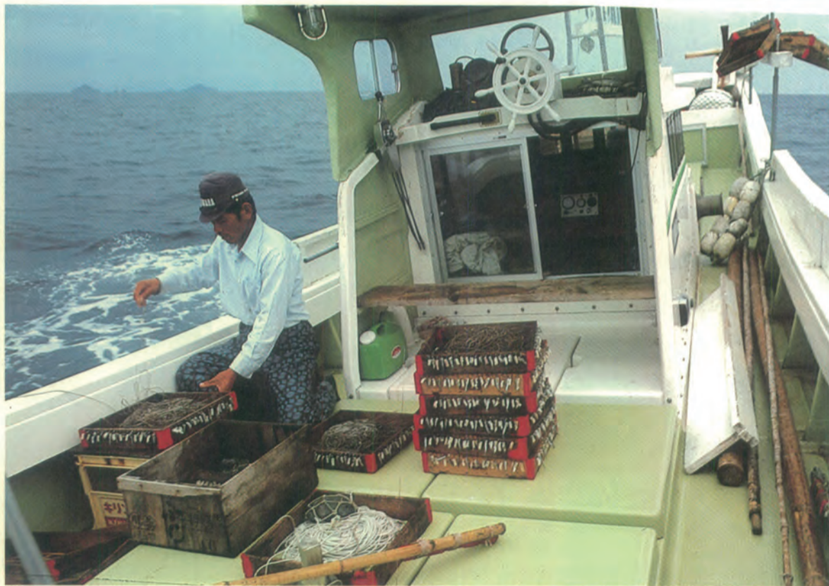
Line casting: The boat is driven forward at 4~5 knots as the line is cast. An automatic pilot is used to control the boat.
