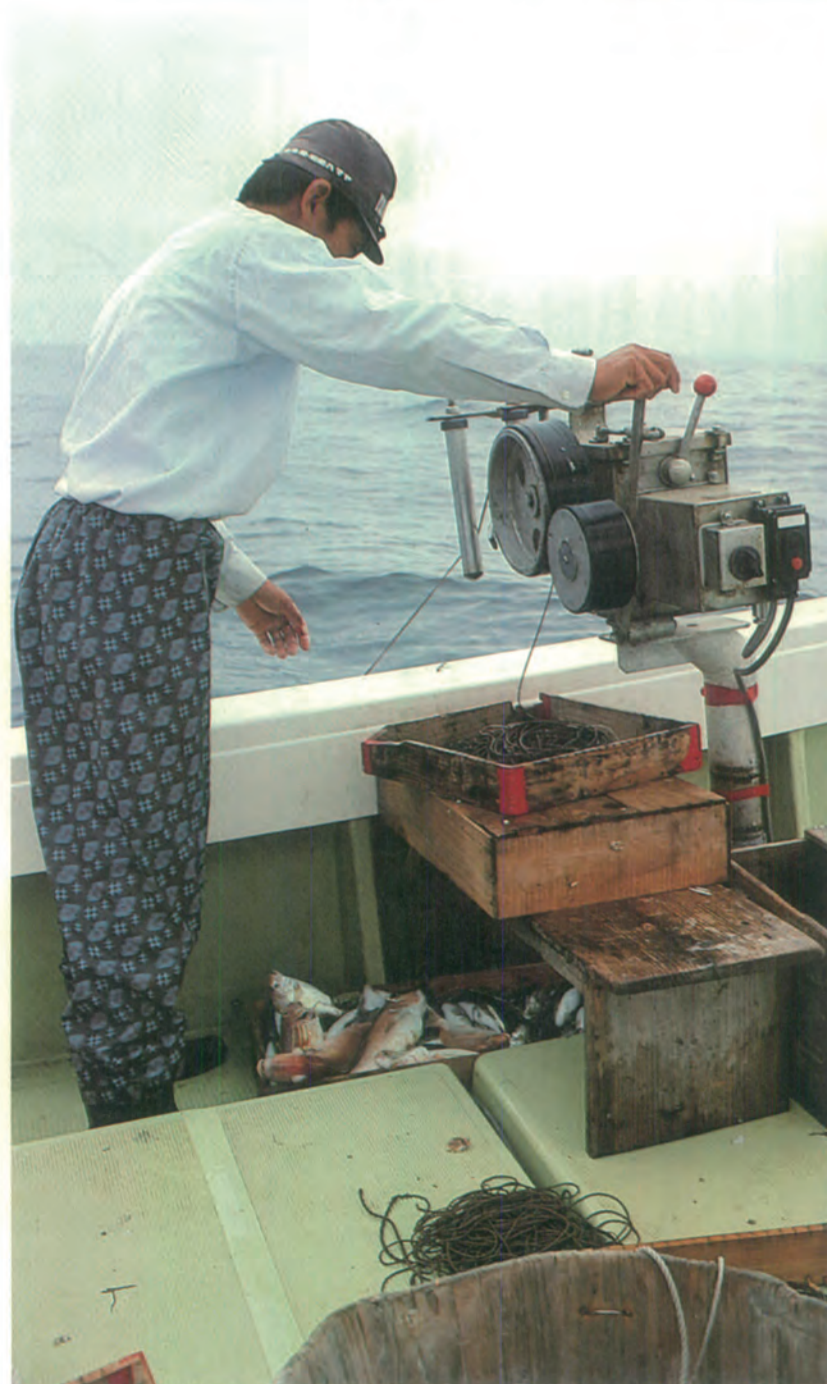
Line hauling: The line is reeled in automatically by a line hauler.
