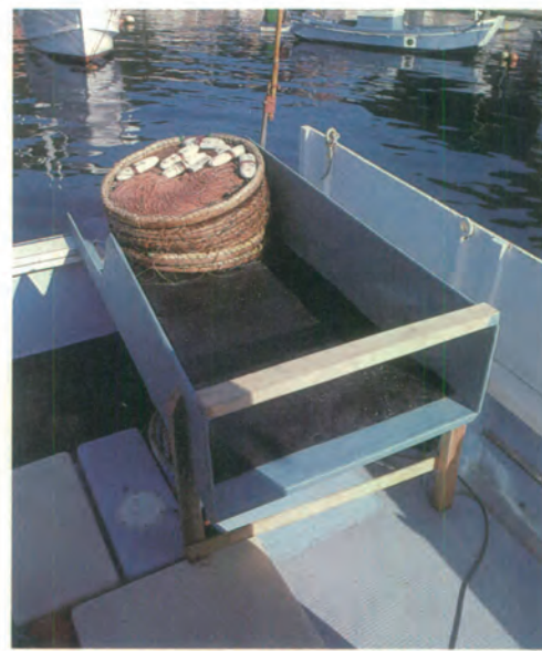
Salmon longline. A line-casting platform is built on the stern of the boat.
