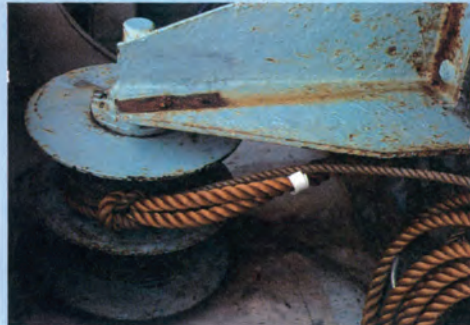
Propeller cover: This covers the propeller when the boat reaches the fishing ground in order to prevent the tow rope or other nets from getting tangled up in the propeller.
