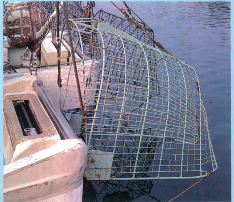
Propeller cover: This covers the propeller when the boat reaches the fishing ground in order to prevent the tow rope or other nets from getting tangled up in the propeller.
