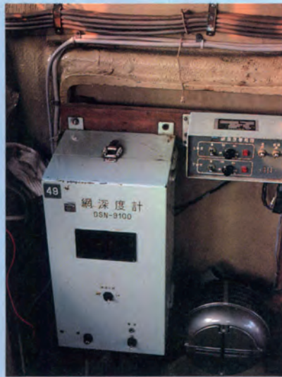
Net zonde transmitter: The component on the right is hung from the center of the grand rope, and the left one is hung into the water from the side of the boat.
