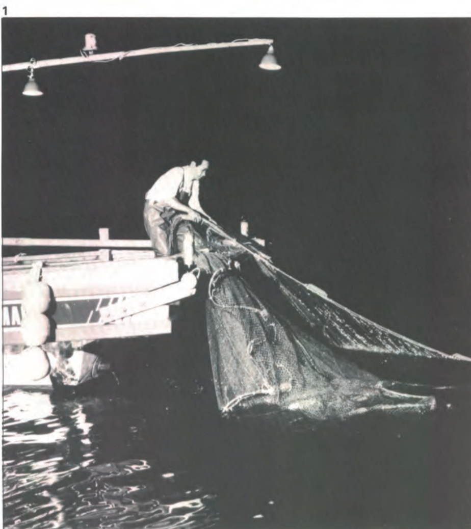
1-4. Net dragging: The bag net (cod end) is grasped by hand, moved to the side from the stern and dragged up onto the deck. Catches are taken out by opening the cod end.
