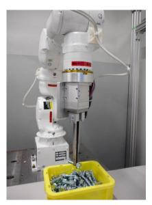
Al Picking by using machine vision
