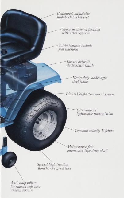
scalp rollers ensure professional-quality results over rough terrain. And with Yamaha's Dial-a-Height™ adjustment system, your preset mowing height is constant, insuring the highest quality of cut.
