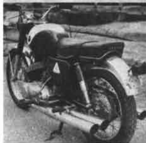
Material was removed from each side of the two center cylinders to retain the standard 90-mm centerline-to-centerline spacing. No overhauling problems have been encountered. The Yamaha YDS-3 looks perfectly standard except for the four exhaust pipes. Engine is now 7.79 in. wider than standard. Engine mounts had to be relocated.
