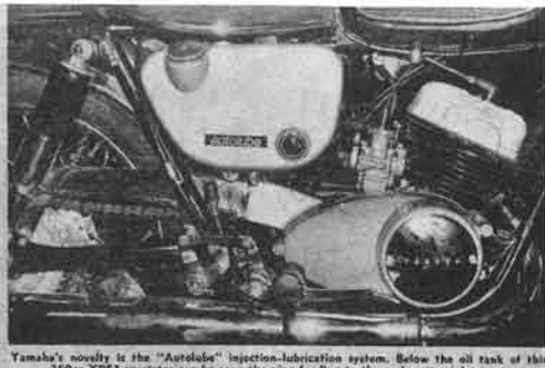
Yamaha's novelty is the "Autolube" injection-lubrication system. Below the oil tank of this 125cc YD153 sportster can be seen the pipe feeding to the carburettor inlet tract.
