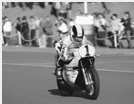
This is the 1978 YZR500 that Kenny Roberts rode to his first world championship title. It was the first YZR500 to mount "Yamaha Power Valve System (YPVS)" for optimized torque characteristics.
