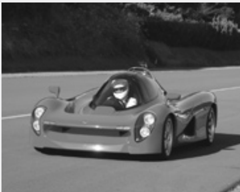
The OX99-11 GP supercar mounts a Yamaha F1 engine in an aluminum chassis hand crafted in the British tradition. Sixteen years after its 1992 debut it is still a thrill to watch.
