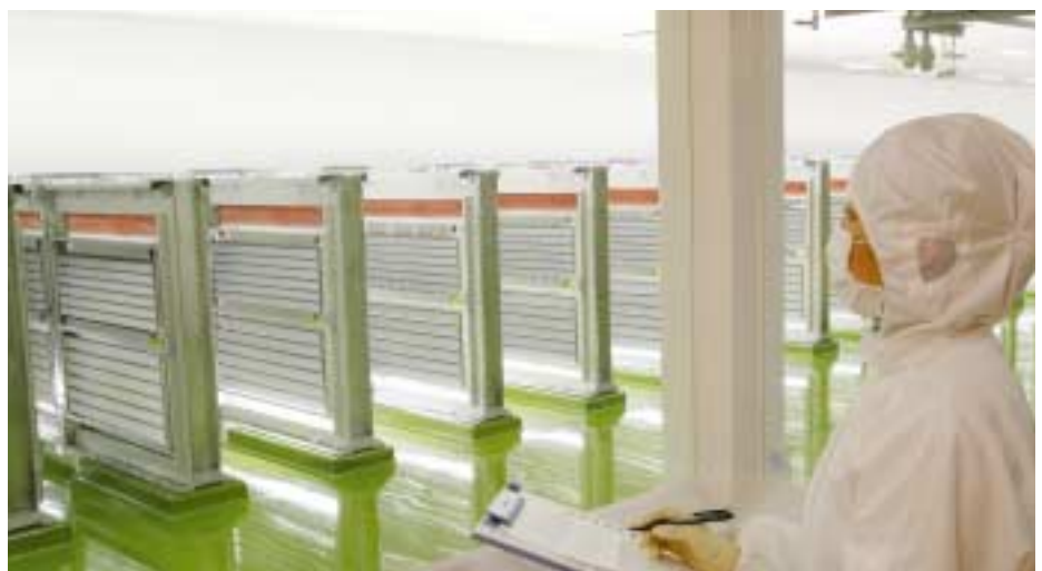
The Yamaha High-Efficiency Bioreactor consists of plates stacked about two meters high and measuring about nine meters in length. Its interior is filled with culture medium, on which a mass of Haematococcus algae floats
