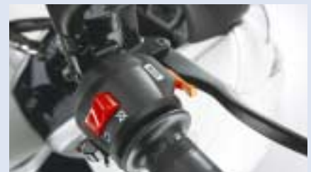
This is the mode switch that enables the new YCC-AT transmission. With this switch on the right handlebar, the rider can choose freely between running modes based on road conditions or rider taste
