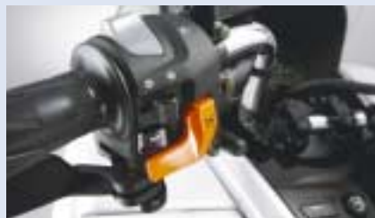
The I-S switch is positioned on the left handlebar and makes it possible to down-shift with a simple touch of the switch
