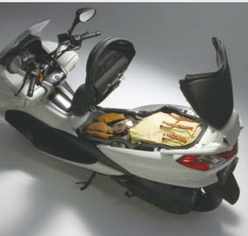
Below the front- and rear-opening seat is a storage space 107 cm in length and with a total volume of 60 liters
