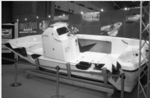
A cut model of the "BAYSPORTS 21" boat built with the FOAMAP construction method to achieve the very highest level of floatability
