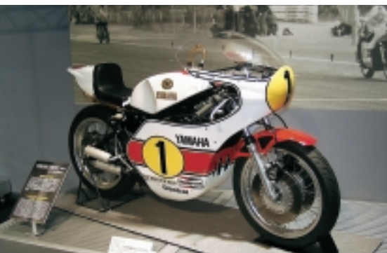
The OW23 was the first YZR with an engine designed specifically for the 500cc class
