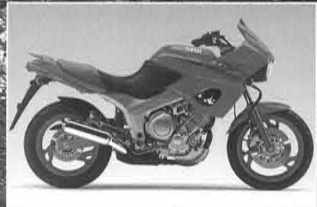
In 1996 the 2nd-generation "TDM850" appeared with a new engine spec and a crank angle changed from 360 to 270 degrees. The 1st and 2nd generation TDMs have sold a total of some 62,000 units in the European market through the year 2000
