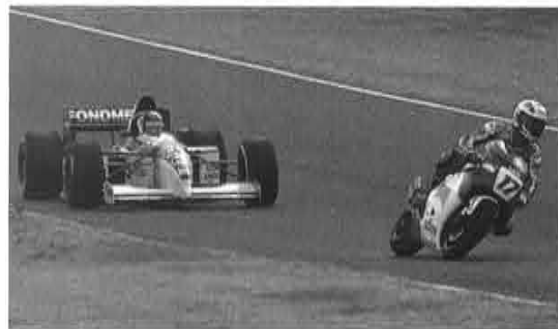
Although the F1 car packs three times the power of the GP bike, the latter has a big power-to-weight advantage
