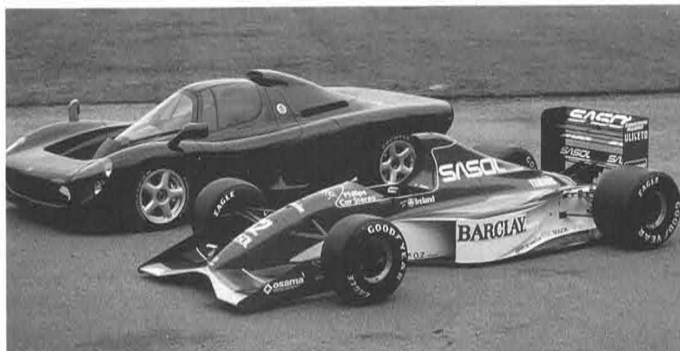
The GP SuperCar is mounted with Yamaha Motor's present F1 engine as its power unit.
