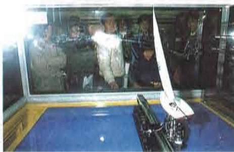
By means of a remote controlled model sailboat, a device shows an interrelation between the wind blowing against sails and resultant boat course.
