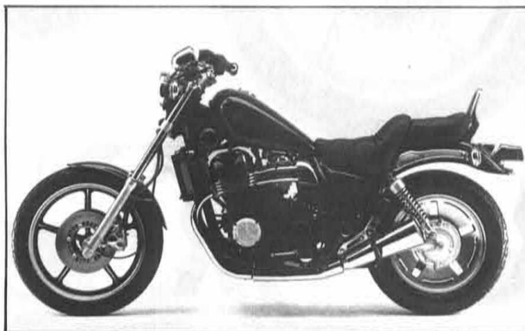
engine width. There's also a newly designed shaft drive for smooth and reliable power transmission. Dual-disc front brakes employ the latest opposed-piston calipers for quickly stopping this Cruiser missile.
