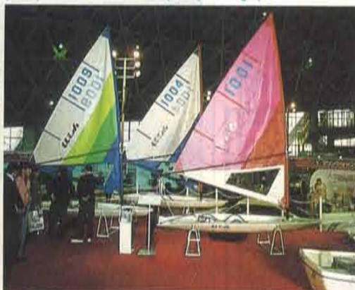
The compact, lightweight "Wish" is a cartopper. It is partly a board sailer and partly a dinghy.
