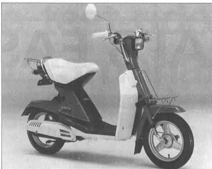
The Pasetta SB50E is an entirely-new sports scooter which was introduced in April of this year. Its attractive and nimble-looking styling appeals to novelty-minded customers. Both with and without an electric starter models are available. The 2.6hp engine and automatic transmission are also featured in this model. With these additions the Yamaha scooter range has been greatly strengthened to gain widespread popularity among both male and female customers.
