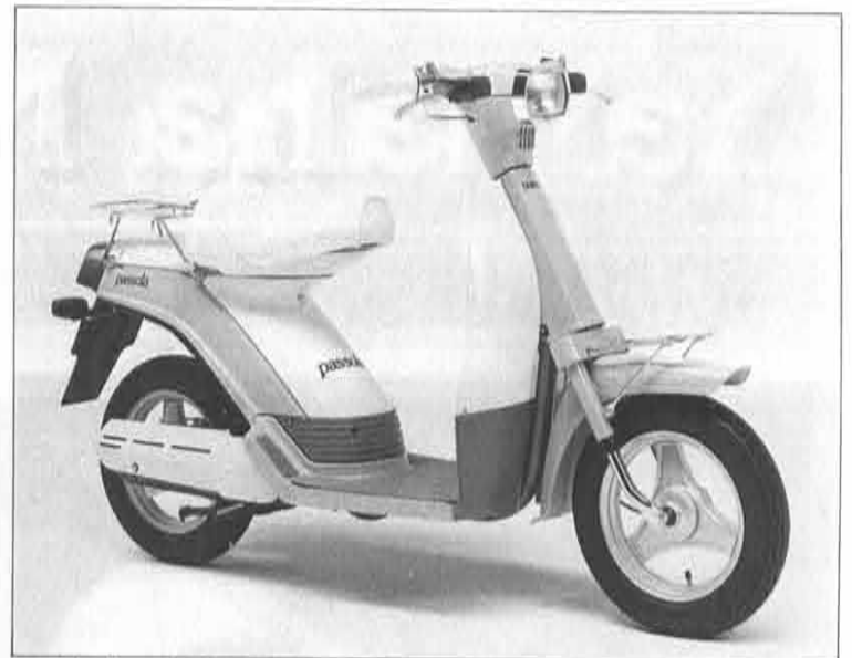
The Yamaha Passola SA50 which was introduced on the market in February 1978, is an up-graded soft bike. Its design concept is similar to that of the S50 but its power output is increased to obtain more riding comfort. The chassis is also enlarged, with both front and rear 2.75-10-4PR tires. The engine delivers 2.8hp and 2-speed automatic transmission operates dependably at all times. The standard model features a kick-starting system but an electric starter type was also marketed in February of this year. Combined total production of the S50 and the SA50 reached the one million mark in Feb. 11 of this year.
