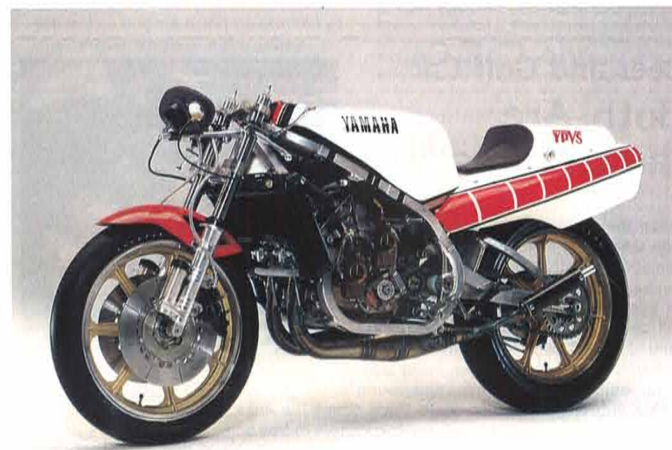
•Engine type: 2-stroke, water-cooled, YPVS, rotary disc valve, square 4 cylinders •Displacement: 499cc •Max. power output: — •Max. speed: — •Ignition: C.D.I. •Lubrication: Mixing (30 : 1) •Clutch: Dry multi-plate •Transmission: 6 speeds •Tire (Front): 3.25/4.00-18 (Rear): 4.30/6.30-18 •Suspension (Front): Telescopic (Rear): Swing arm (with Monocross system) •Brake (Front): Double disc (Rear): Single disc
