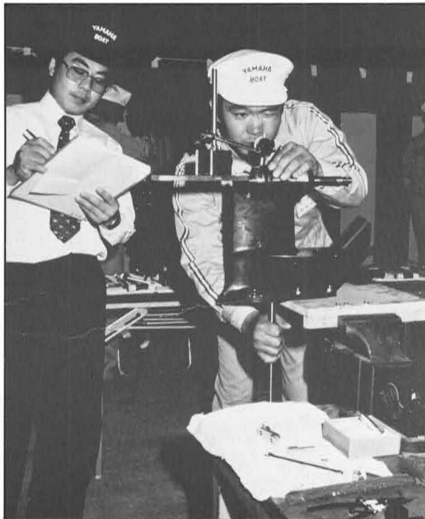
He is carefully taking dial gauge readings.
