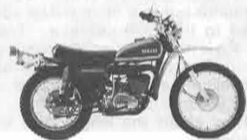
'73 model with a raised front fender and thermal flow rear suspension
