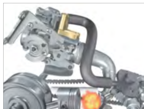
* YMJET-FI = Yamaha Mixture Jet-Fuel Injection. A fuel injection system employing an auxiliary air intake passage in addition to the main passage, to provide an "air assist" for more efficient mixing of the air and fuel that helps improve fuel economy in the practical use range.
